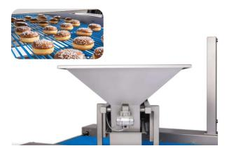
Enrobing and Dipping Section Cover: The dipping machine can be equipped with a heated cover to prevent a loss of temperature and dirt from falling in. This cover consists of a stainless-steel frame with Lexan windows, which splits into two separate covers placed over the dipping section. Covers can be removed manually for cleaning.
